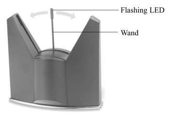
(a) The tip of the wand moves with simple harmonic motion as it sweeps through a distance of 10.0 cm from one end to the other.
